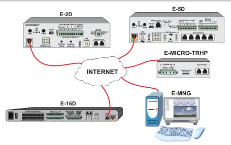
How to connect and control up to 3,000 E-2D/5D/16D, E-MICRO-TRH(P), and E-1W(P) units via Ethernet
