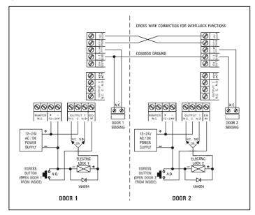
An inter-lock system needs two door controllers. This application example uses two DK-9522 with simple cross wire connection on their "Output I Inhibit" and "Inter-lock Control Output" terminals. It is necessary to link up the "(-) GND" terminals of the two keypads as common ground to achieve the inter-lock logical functions.
