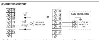
The Duress Output switches to (-) ground when duress code is entered. You may use it to turn ON an LED lamp and/ or a small buzzer to notify a guard; or connect it to a 24 hour Normally Open protection zone of an alarm system.
