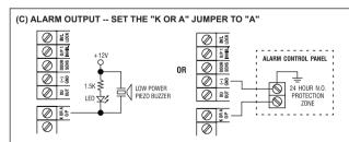
The Alarm Output switches to (–) ground in door forced to open or the door open after Egress Delay, You may use it to turn ON an LED lamp and/ or a small buzzer to notify a guard; or connect it to a 24 hour Normally Open protection zone of an alarm system. See Location 80 and Location 91 for more information about these functions.
