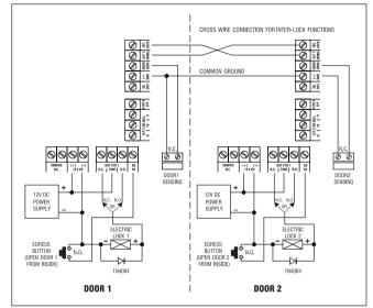
An inter-lock system needs two door controllers. This application example uses two DK-2822 with simple cross wire connection on their "Output 1 Inhibit" and "Inter-lock Control Output" terminals. It is necessary to link up the "(–) GND" terminals of the two keypads as common ground to achieve the inter-lock logical functions.
