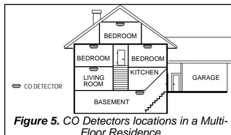
Figure 5. CO Detectors locations in a Multi-Floor Residence
