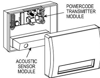
Figure 2. Module Identification
