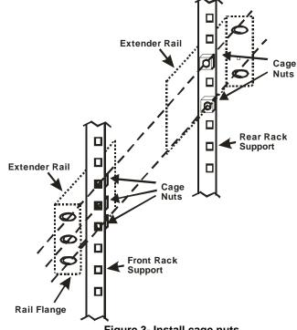
Figure 3- Install cage nuts
