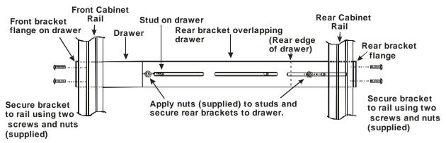
Figure 1- Mount RACKMUX to a standard rack
