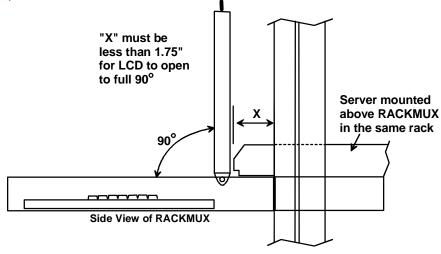
Figure 8- Position RACKMUX with clearance to open
