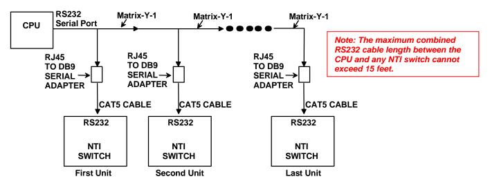
Figure 16- RS232 connection with Matrix-Y-1 cable
