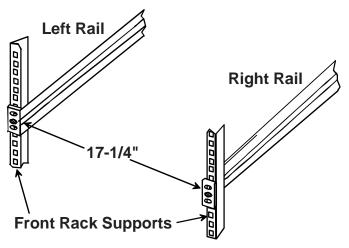
Figure 5- Adjust distance between rails
