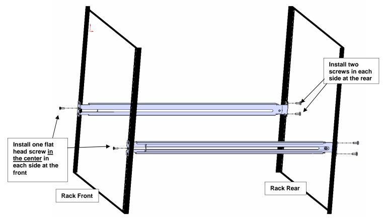
Figure 4- Install rail assemblies
