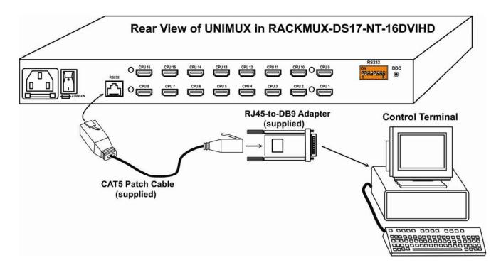
Figure 12- Connect RS232 control terminal
