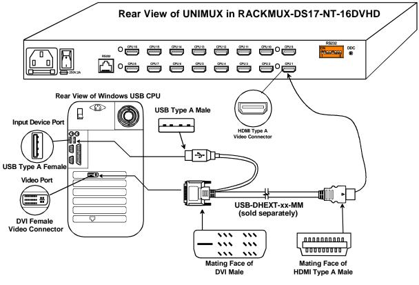
Figure 10- Connect each CPU
