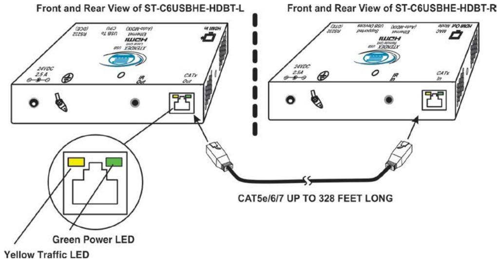
Figure 3- Connect CATx cable
