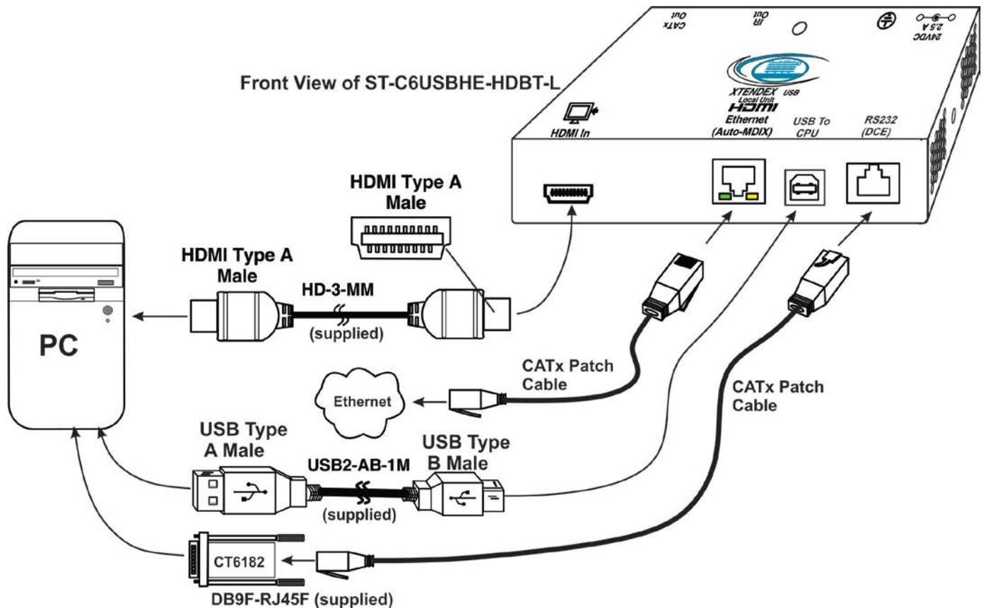
Figure 1- Connect the XTENDEX Local Unit to the computer
