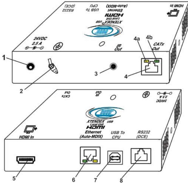
Front and Rear View of ST-C6USBHE-HDBT-R
