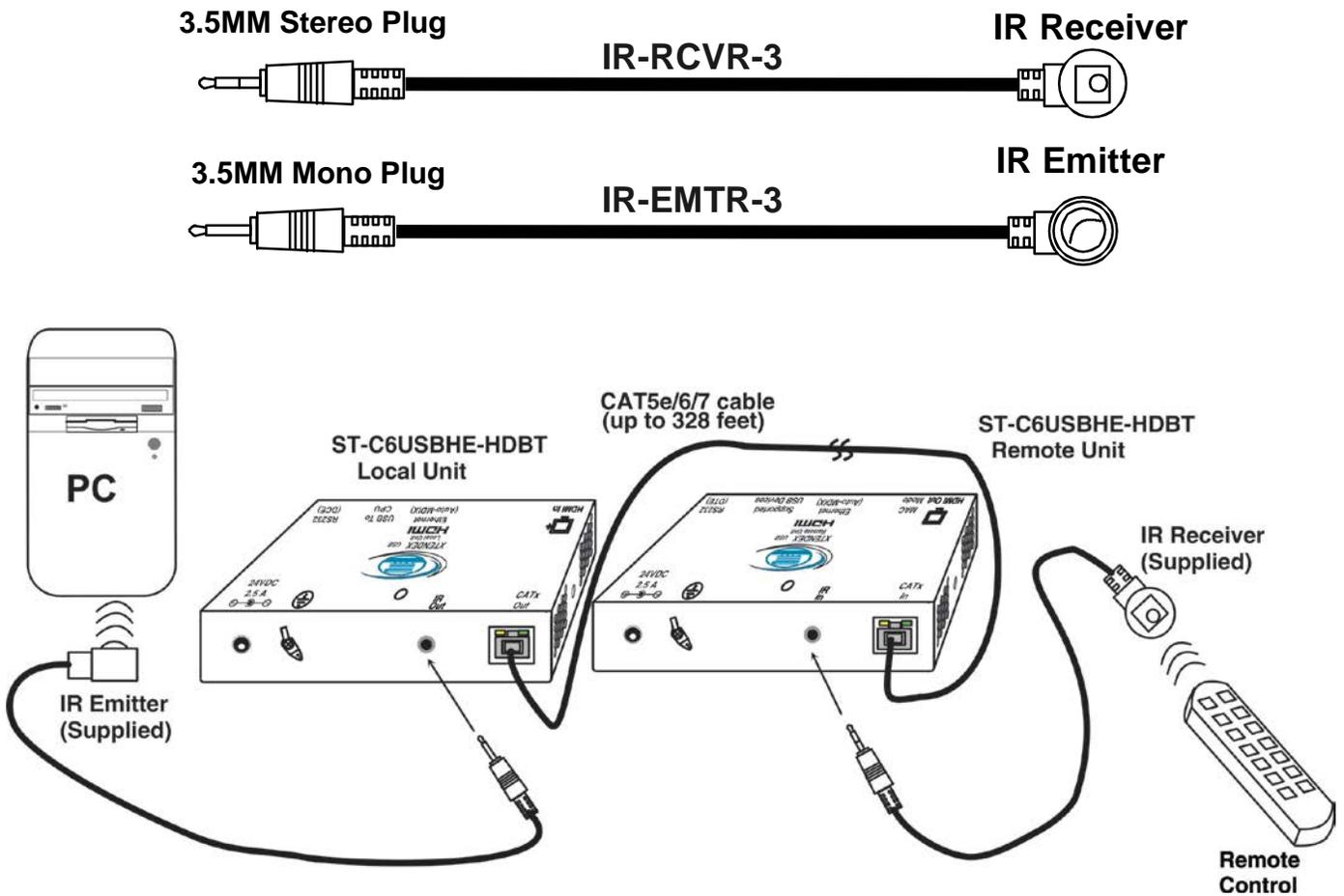
Figure 5- Connect IR Emitter and Receiver
