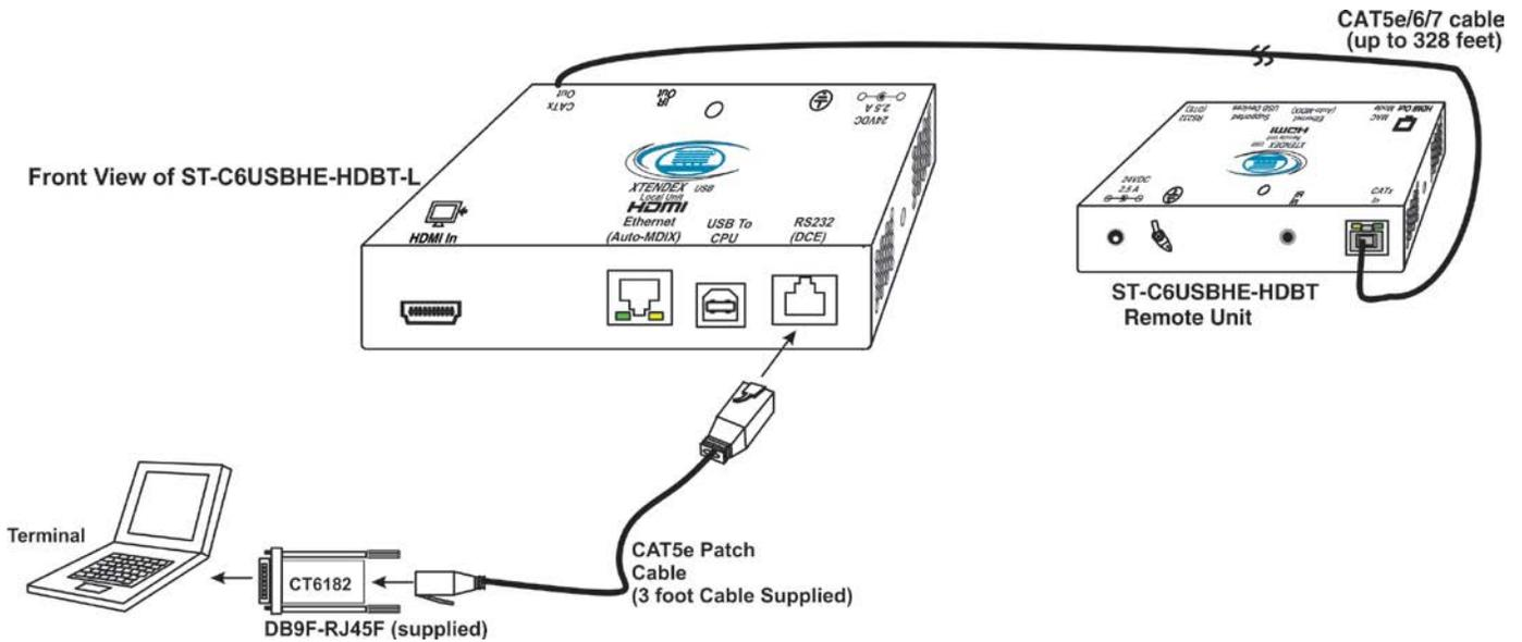
Figure 7- Connect PC for firmware upgrade
