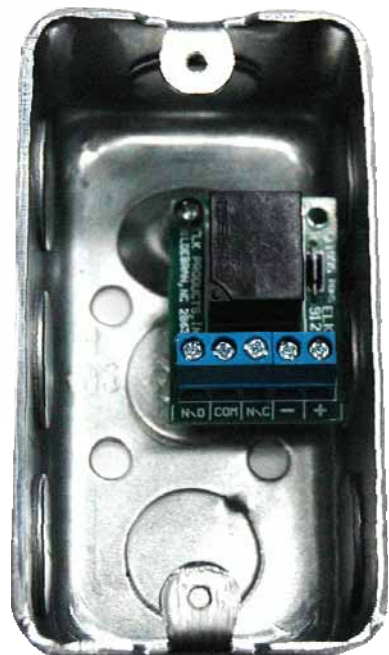
The Relay Kit includes a relay circuit board mounted inside an electrical enclosure. (Cover plate not shown)
