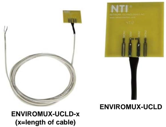
ENVIROMUX-UCLD is an Under-Carpet Leak Detector for sensing the presence of water under carpeting or rugs in an environment where knowing moisture is present is desired. When connected to an ENVIROMUX-SEMS-16(U), ENVIROMUX-MINI-LXO, ENVIROMUX-2D, ENVIROMUX-5D or ENVIROMUX-16D Enterprise Environment Monitoring System (SYSTEM) the sensor can be used to alert users as to the presence of water where it would otherwise be hidden.
