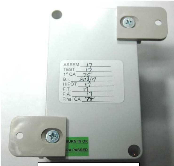
Brackets and screws installed.
