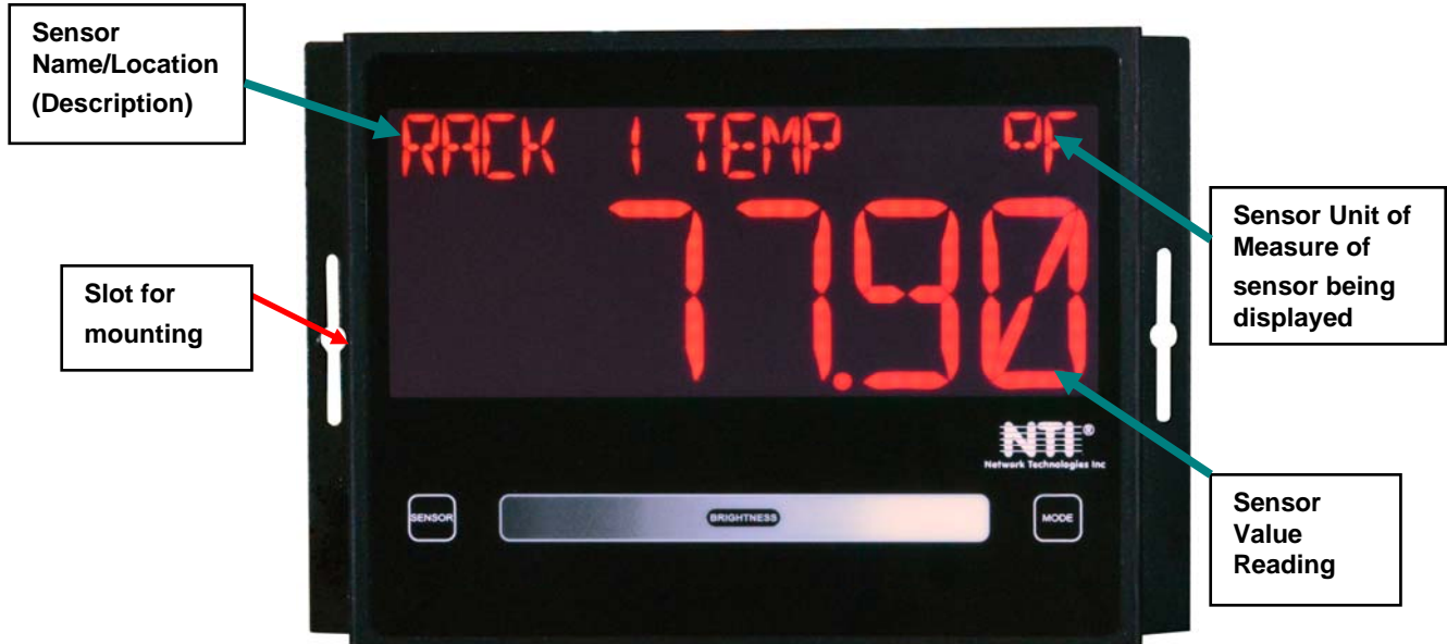
Figure 8- E-PLSD Programmable LED Sensor Display
