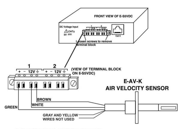
E-S5VDC WITH E-AV-K CONNECTED
