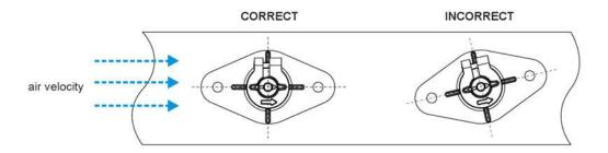
The mounting flange allows for an infinite variation of the depth of the sensor probe. It is important to ensure that the sensor head is completely submerged into the flow.
