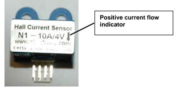
**Installation Note:** When placing a split core hall effect sensor (i.e. E-AMP100-SC12) around a conductor, make sure the sensor core is large enough to be placed completely around the conductor and is closed in order to sense current properly.
