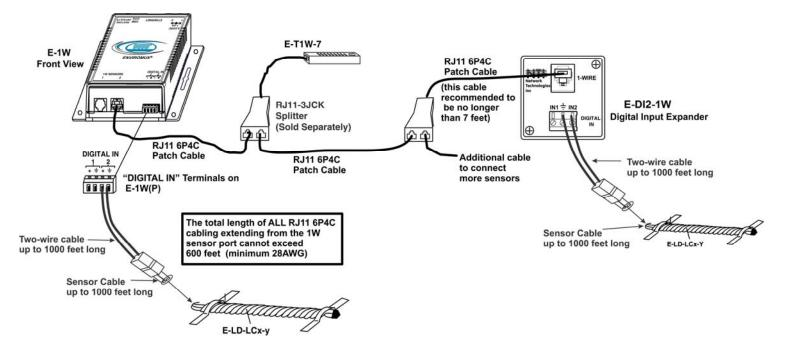
Sensors connected to the E-DI2-1W will be listed under "External Sensors" on the Summary Page in the web interface but will be configured the same as any other digital inputs. For more information on configuring sensors, see the E-1W product manual.
