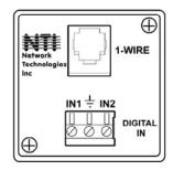
Contact sensors and liquid detection sensors can be connected to the "Digital In" terminals on the E-1W. Another way to connect these sensors is through an E-DI2-1W Digital Input Expander. The Expander provides a way to not only increase the number of these sensors that can be connected, but also to add distance these sensors can be placed away from the E-1W.
