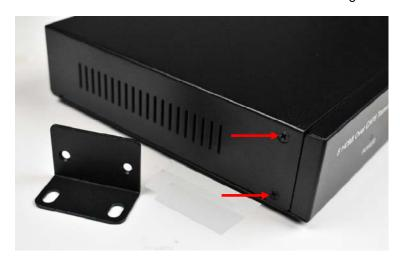
Remove the screws, place the ear, and reinstall the screws.
