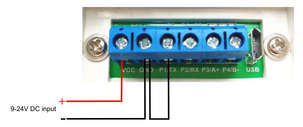
This wiring method is an example of how to play all sound messages automatically in a loop when it's powered ON. The connections must be made prior to applying power. In addition, to achieve this function, the trigger mode in the configuration file must be "3".
