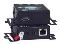
The XTENDEX® ST-C64K-300 4K HDMI Extender transmits uncompressed digital 4Kx2K HDMI signal and IR up to 300 feet over a single CATx solid cable. Each video extender consists of a local unit that connects to an HDMI source and a remote unit that connects to an HDMI display.
