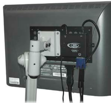
Remote unit mounted to the back of a flat panel monitor using ST-C5MK-VESA mounting kit
