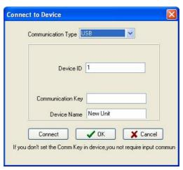
**Device ID, Communication key** and **Device Name** is the same configure as RS232/RS485.
