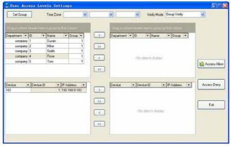
2. Select a user and the applied device, the using time zone and the verification style, and click [Access Allow] button.
