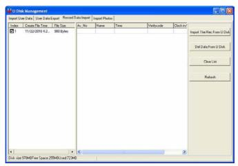
Click [Import the record from U disk], then the system import the data. When it has finished, all records will move to the buffer area.
