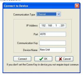
**IP Address:** The default IP address is 192.168.1.201. Please input the IP address of the device you want to connect.
