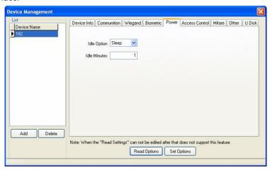
Firstly, read the parameter of [Power], modify the state of [Idle Setup] and minutes of [Idle Time], then click the [Set Options], and restart the device to complete setting.
