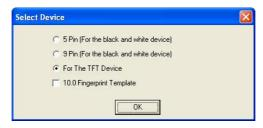
3. After that, click **[OK]** button, the system will automatically search the user data and load it into the system from the U disk. If there is a new use, the data will show in green color. In the list, the records with red color indicate that these records do not synchronization with the data in the software.
