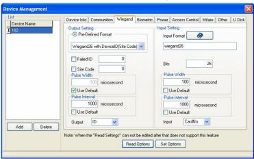
Wiegand Setting includes Wiegand output and input setting.
