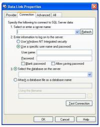
Confirm the server name for storing this database, information for logging on this serve, and the database name. After run test connection successfully Click [**OK**] button to complete settings
