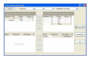
8. After users and device selecting, click on [Access Allows] button, the group time zone that using by user in the critical periods will be assign to the selected devices. After distribution is successful, prompt will appear shown as following
