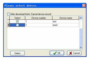
Select the device and click **[OK]** to finish the download process. If you select [After download Finish, Cancel device record], the system will delete the device record when downloading complete.
