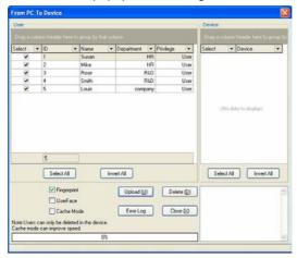
**Upload**: Based on your need, select the user and an uploading FP device, click [**Upload**], it is able to upload user's data to the defined FP device, it is better to select [**Fingerprint**] and [**User Face**] in the normal condition. If the information needs not to modify, it is no need to choose it.
