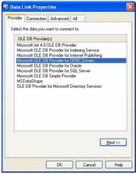
Click button, can select the database file, the default name is att200.mdb, according to real condition to renew setup of the database connection.
