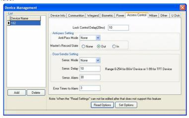
**Lock Control Delay:** Apply to determine unlock hour, the minimum measured unit is 20 ms, in the normal condition that is 100-200 ms.
