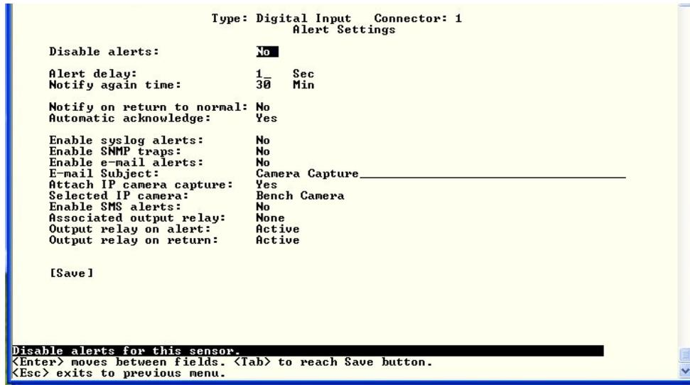
Figure 6- Digital Input Alert Settings
