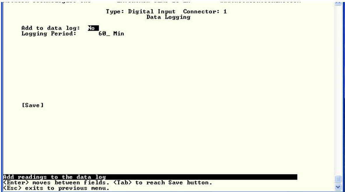
Figure 7- Data Logging for Digital Input Sensors
