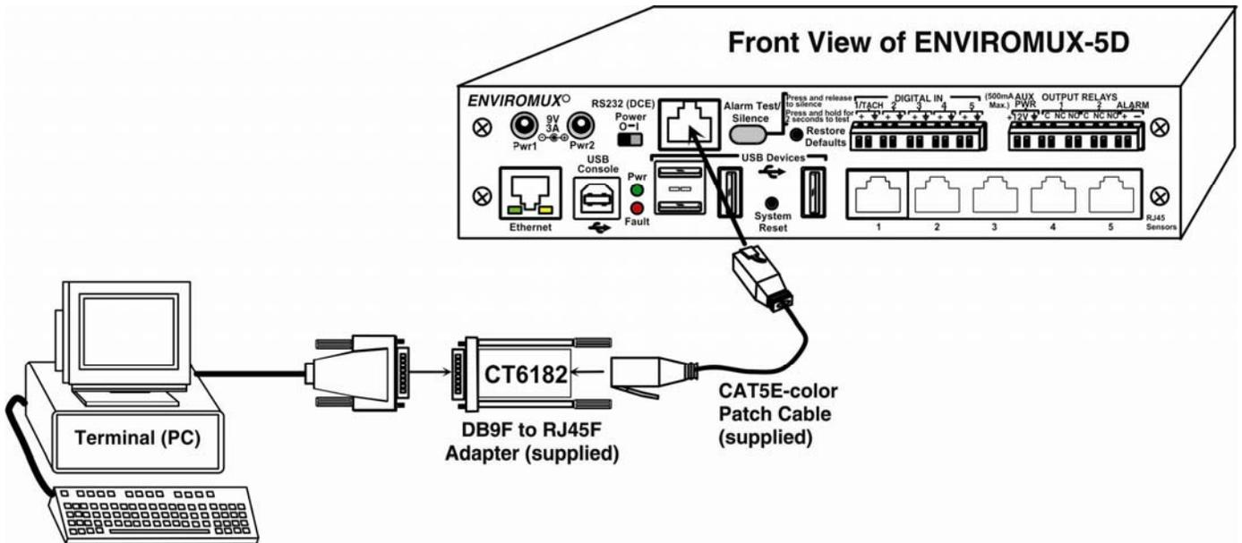
Connect a terminal for direct RS232 serial communication
