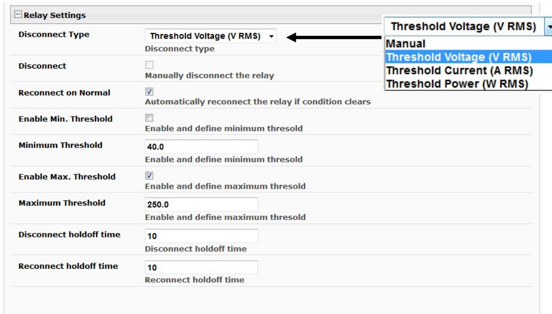
Figure 10- ACLM-P Spike Threshold and Relay Settings
