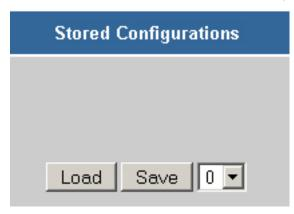
Note: This will save the currently <u>active</u> configuration on the VEEMUX. If changes have been made in the web interface without first pressing the Submit button, those changes will not yet be part of the <u>active</u> configuration.
