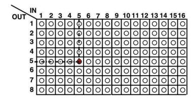
Figure 5- LED Matrix showing input 5 connected to output 5
