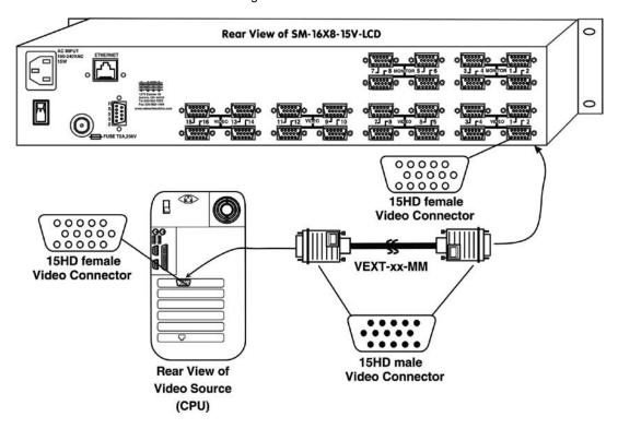
Figure 1- Install Video Source Cables
