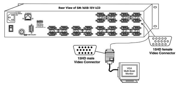
Figure 2- Connect a monitor to the VEEMUX
