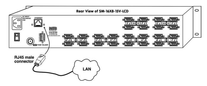
Figure 4- Connect the LAN to the VEEMUX
