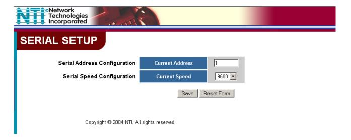
Figure 12- Web interface Serial Setup page
