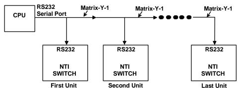
Figure 6- RS232 connection with Matrix-Y-1 cable
