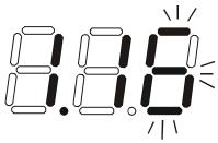
With the desired port number selected, point the IRT at the switch/receiver and press the "OUT" button to transmit the selection and make the change. The blinking number in the LCD will stop blinking. An LED on the receiver will illuminate.
