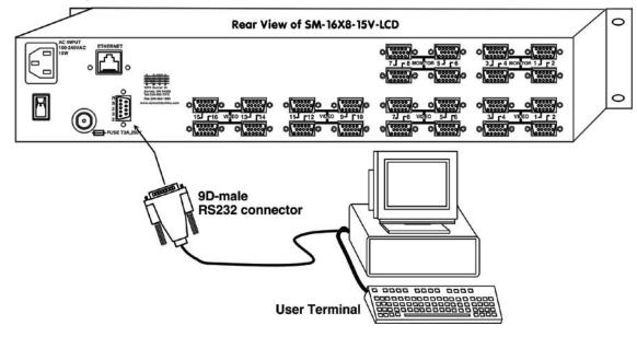
Figure 3- Connect user terminal for RS232 control
