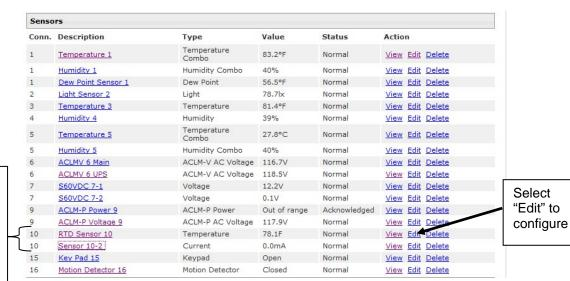
An RTD sensor is connected to one input on the current sensor, the second input has not been configured.
