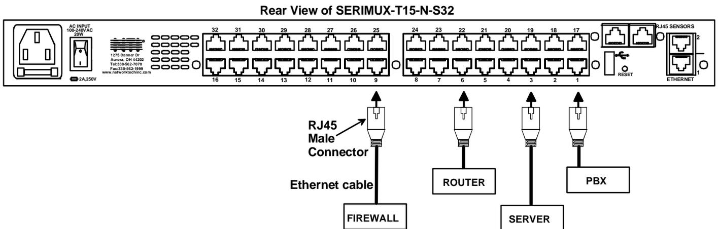
2. Connect the power cord to the IEC connector.
