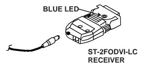
Figure 3- Connection of the power adapter to the receiver
