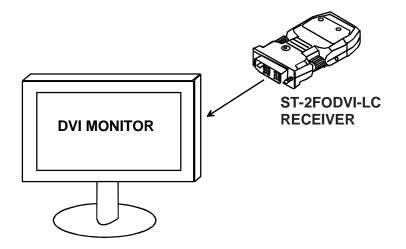
Figure 6- Connection of the receiver to the display
