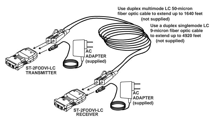
Figure 4- Connection of optical fibers
