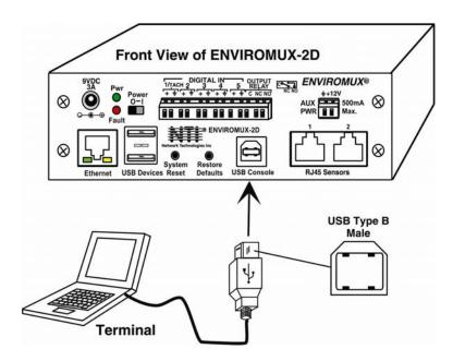
Figure 9- Connect terminal to USB Console port
