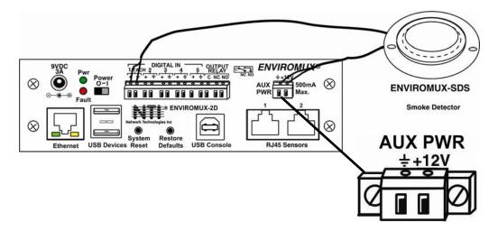
Figure 7- Use AUX PWR to supply 12VDC
