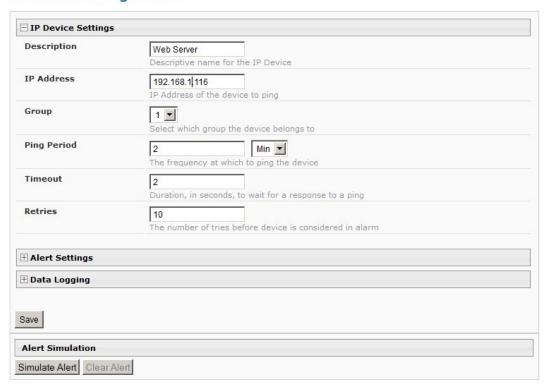
Figure 28- IP Device Configuration page
