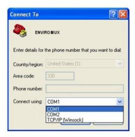
Figure 11- Configure COM port in HyperTerminal
