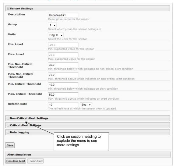
Figure 20- Sensor Configuration page
