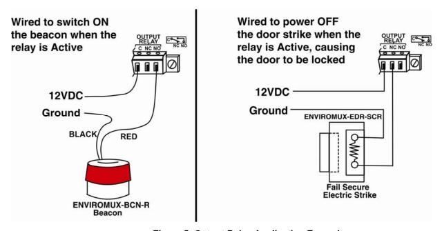
Figure 5- Output Relay Application Examples
