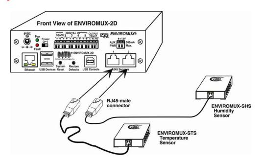
**Figure 1- Connect Sensors**
