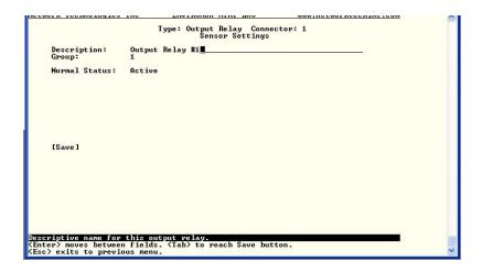
Figure 91- Text Menu- Output Relay Settings
