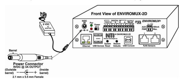
Figure 12- Connect the AC adapter and power-up
