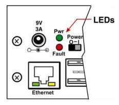
Figure 13- LEDs on front of ENVIROMUX
