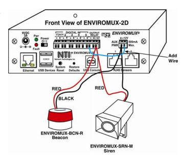
Figure 6- Control multiple devices from relay
