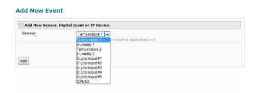
Figure 57- Sensor to be used for a predefined event
