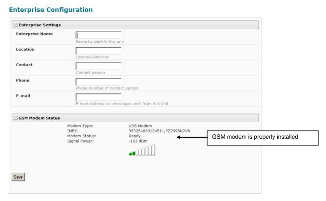
Figure 42- Enterprise Configuration- Modem Status "Ready"
