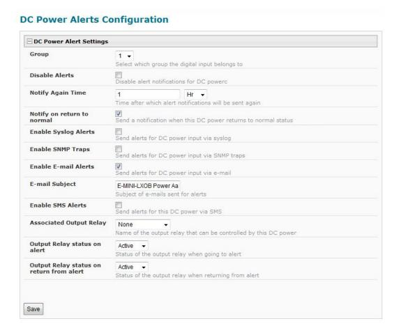
Figure 38- DC Power Alert Configuration
