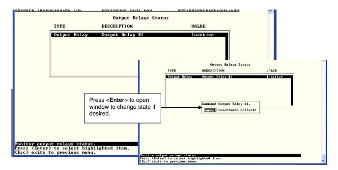
Figure 75- Text Menu- View Output Relay Status
