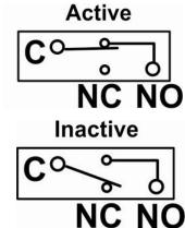
Figure 32- Output Relay Status
