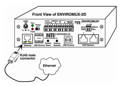
Figure 8- Connect ENVIROMUX-2D to the Ethernet
