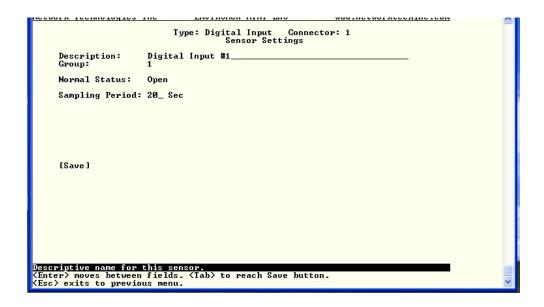
Figure 82- Digital Input Sensor Settings Menu
