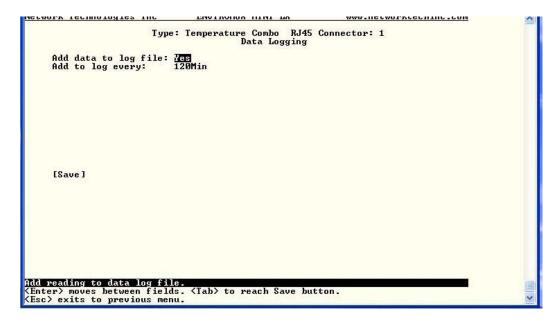
Figure 80- Text Menu-Sensor Data Logging
