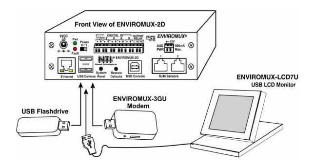
Figure 14- Connect a USB device
