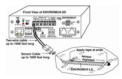
Figure 3- Secure liquid detection sensor with tape
