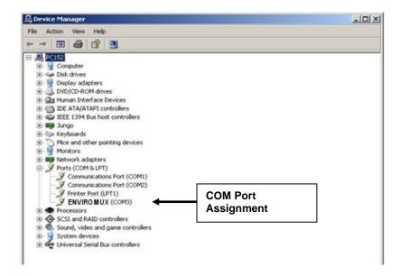
Figure 10- COM port assigned to ENVIROMUX
