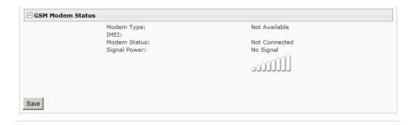
Figure 43- No Modem Installed
