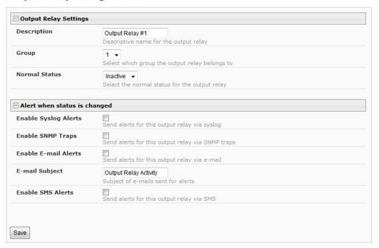
Figure 34- Configure Output Relay
