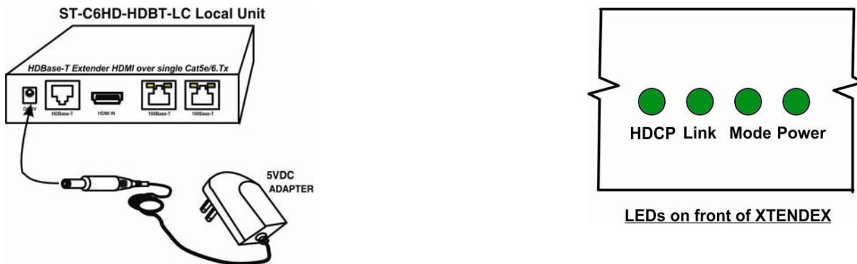
Figure 4- Connect the AC adapters to the Remote Unit and the Local Unit
