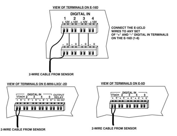
CONNECT THE E-UCLD WIRES TO ANY SET OF "+" AND "  $\stackrel{\leftarrow}{\div}$ " DIGITAL IN TERMINALS ON THE E-MINI-LXO, E-2D OR E-5D
