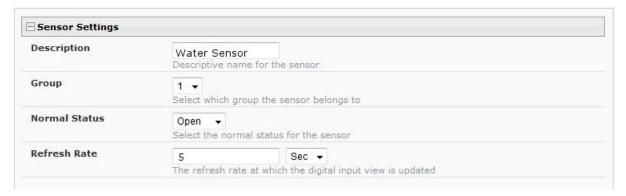
Figure 1- Sensor configuration page from E-2D/-5D/-16D
