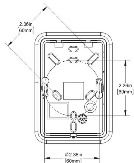
**Fig. 4:** 60mm mounting base dimensions
