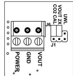
Fig. 7: J1 Set for 0 to 5 VDC Output
