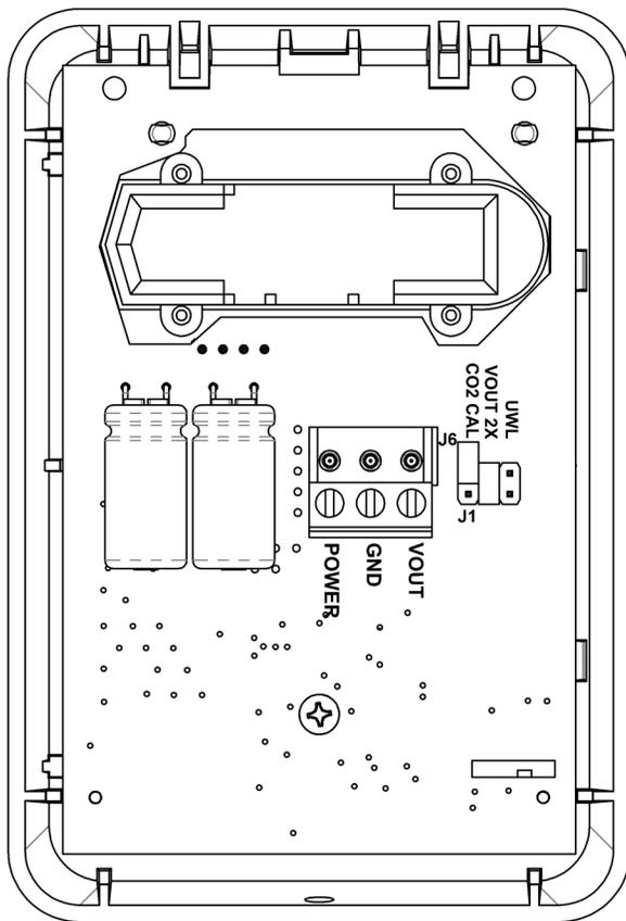
Fig. 5: Circuit Board
