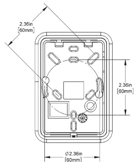
**Fig. 4:** 60mm mounting base dimensions
