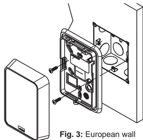
**Fig. 3:** European wall box mounting with 60mm base
