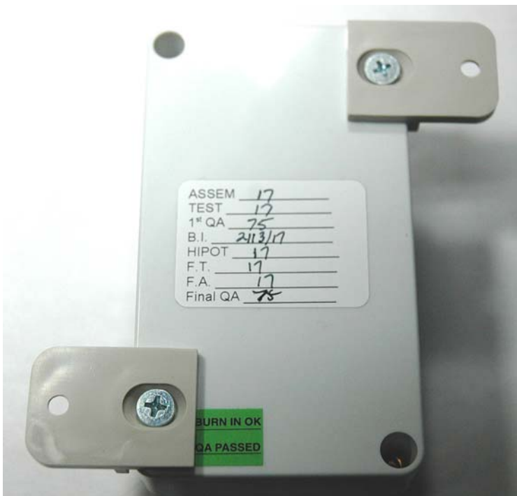
Brackets and screws installed.
