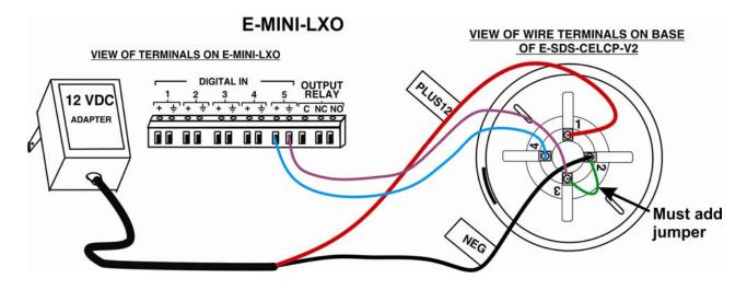
Wired using this method the smoke detector must be manually power-cycled in order to reset it when it goes into alert.
