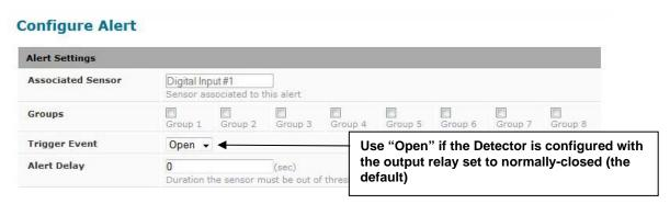
**Example of sensor configuration in E-MICRO-T(RHP)**
