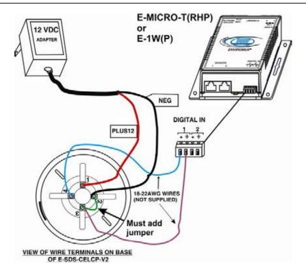
To wire your own CATx patch cable to an E-SDS-CELC-V2 sensor, follow the wiring instruction below.
