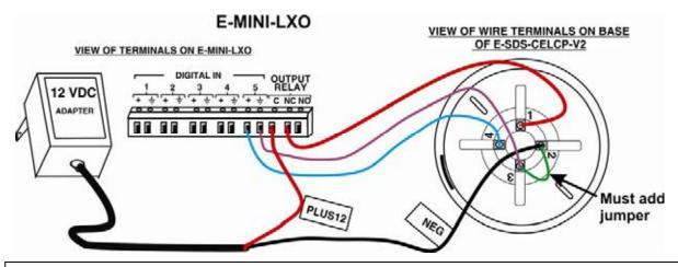
Wired using this method the smoke detector can be power-cycled through the web interface when it is in alert. Make sure that no sensors are configured to activate the output relay when in or out of alert. (See page 9)
