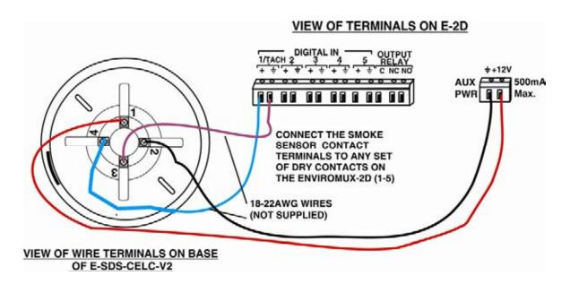
Model E-SDS-CELCP-V2 can be used when a 12VDC power supply is not available on the SYSTEM. (For example, E-MICRO-TRH(P), E-1W(P) and E-MINI-LXO do not include terminals to provide 12VDC power to sensors)
