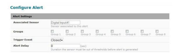
Example of alert configuration in E-MICRO-TRH(P) or E-1W(P)
