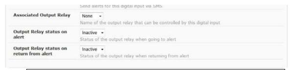
Make sure the ENVIROMUX Output Relay status for both fields in all sensor configurations is set to "Inactive" if the output relay is used to power the smoke detector.
