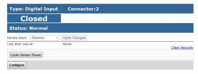
When the sensor is in an "Alarm" state, the Status screen will indicate the switch is "Open".
