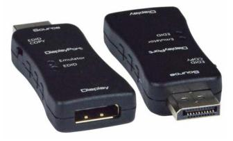
The DP4K-EDID-EMLTR DisplayPort 1.2 EDID Emulator copies the EDID of the desired DisplayPort display and connects directly to the DisplayPort source to ensure that the EDID is not lost in connections between devices such as splitters and extenders.
