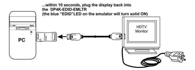
Note: If the emulator needs to be reset back to its default EDID resolution of 1920x1080p, switch the EDID/COPY switch to "EDID".
