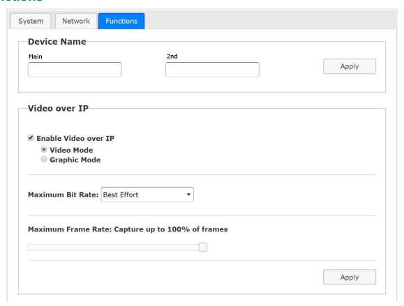
Figure 1- Video over IP Functions for the TX (Local Unit)
