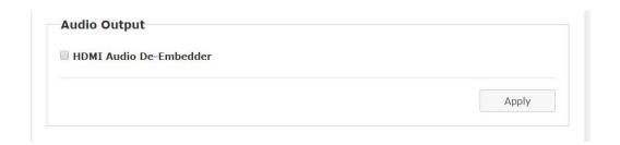
Note: If any 3.5mm audio ports on the TX or RX are used, audio will not be routed through the HDMI cable at the RX.
