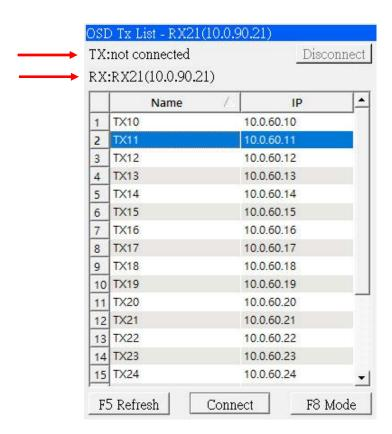
**To connect to a Tx:** Select a Tx using a mouse or ↑↓, then click the **Connect** button to make a connection.
