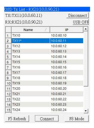
To Start/Stop the USB connection with the current Rx USB over IP: Press "USB ON/OFF" button.
