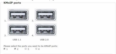
Enable the port #1, 2, 3, 4 for the device to be linked with the TX's K/M over IP HID emulation port. **Default Port 1 and 2 KMoIP Enabled.**
