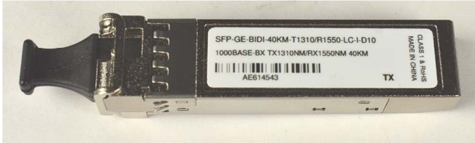
Transceiver for the Transmitter (Top View)
