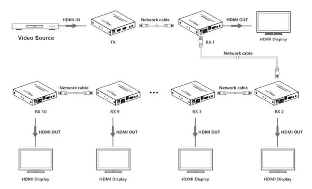
Note: To ensure the quality of the signal transmission, please use a network cable within 70 meters when Remote Units are cascaded.
