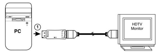
2. Unplug the cable from the "Display" port going to the monitor.
