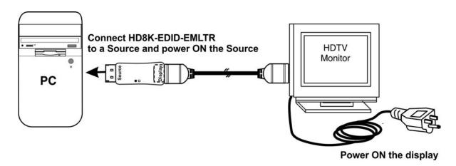
2. Plug the HDMI male ("Source") connector of the HD8K-EDID-EMLTR emulator into the video source. Power ON the video source (if not already ON).
