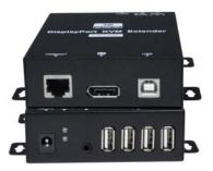
The XTENDEX® ST-C6USBDP4K-328 4K DisplayPort USB KVM HDBaseT Extender transmits uncompressed digital Ultra-HD 4Kx2K 30Hz 4:4:4 DisplayPort signal, transparent USB, and RS232 up to 328 feet over a single CATx cable using HDBaseT technology. Each extender consists of a local unit that connects to a computer, and a remote unit that connects to a UHD DisplayPort display and four USB 2.0 devices.
